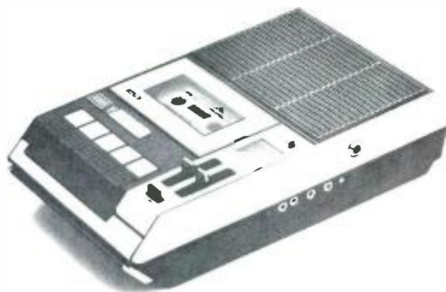
The Variable Speech Control Co. Model A6. The speed slide control has markings for a range of 0.5 to 2.5 times normal.
