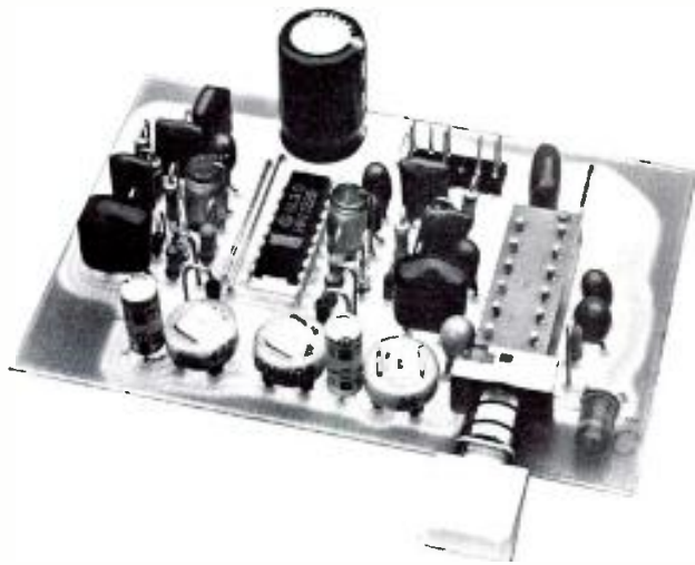
Figure 6. A printed circuit assembly showing additional components required for Dolby f.m. decoding.
